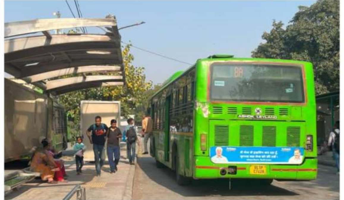
Buses do not stop in alignment with the platform for level-boarding and alighting
