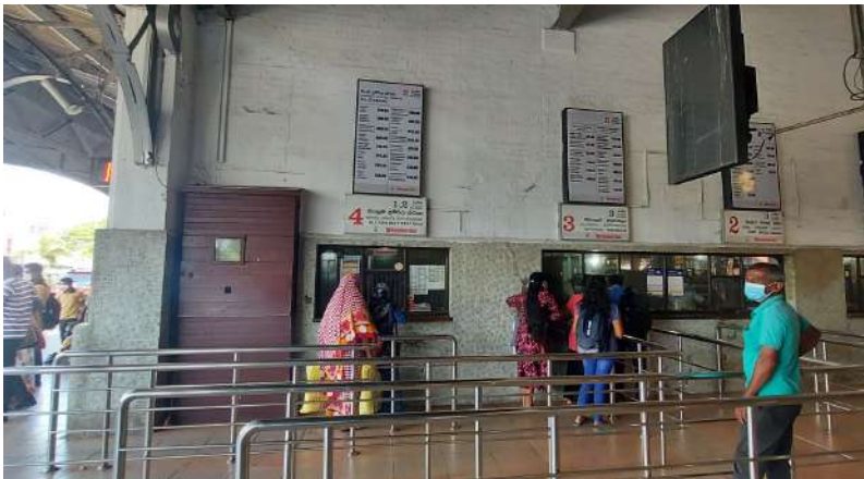
Image showing multiple ticket counters at the Fort station, and they are supported with real-time information. But the handrails are placed too close to each other for a wheelchair to pass through.
