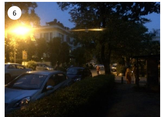
4 5 6 The above photographs show the Lighting levels in Jor Bagh residential area. The high height of the light fixture results it in being obstructed by the foliage. As a result, dark shadows are cast on the footpath making the area poorly lit. Trees should be regularly pruned to prevent this from happening. Also since the lights are installed only on one side of the road, the other side remains poorly lit. Streetlights should be installed on both sides with their position being staggered such that both sides of the road are brightly lit.
