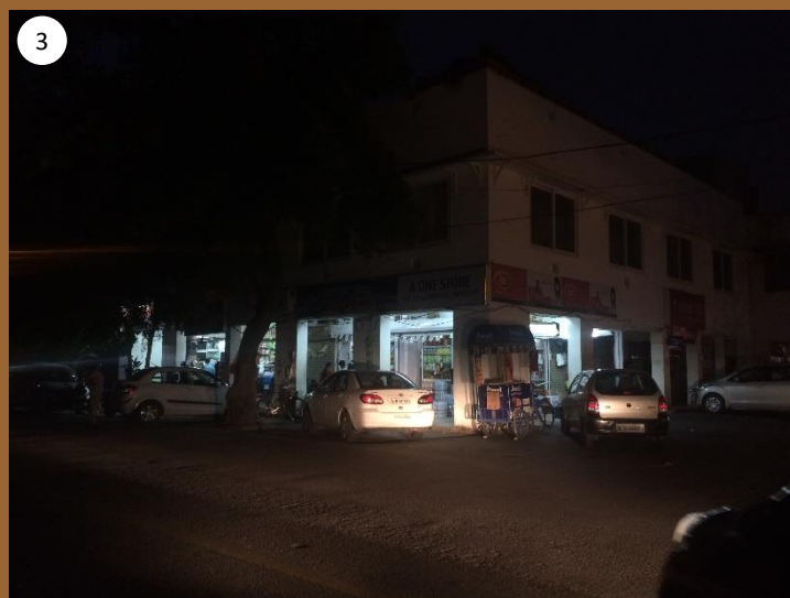
3 Jor Bagh Colony Market. The lighting around the market in the parking area was found to be inadequate with the illumination being primarily from the shops. Streetlights should be installed all around the market such that the abutting area is also brightly lit.
