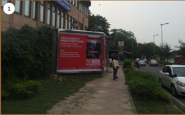
1 Outside Jor Bagh Metro Station. No streetlights are located along the footpath here. Illumination is from the metro station exit and the streetlights along the main road. Pedestrian scale streetlights should be installed along the length of the footpath.
