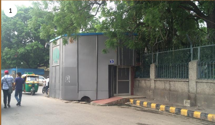
1 Along Aurobindo Marg, the footpath ends abruptly at the Public Toilet. The footpath should be continuous throughout the perimeter of the Public Toilet. The ramp should connect the road with this footpath.
