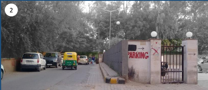
The rear entry of Dilli Haat has a Parking Area. The edge of Dilli Haat does not have a footpath and the one along the Parking is too narrow and too high. The vehicles should not be allowed to park on-street in this area. A proper footpath with tactile paving and ramps needs to be constructed. The boundary wall too should be demolished and be replaced by a Grill to ensure visual connectivity. The gate and piers serve no purpose and should be demolished as well.
